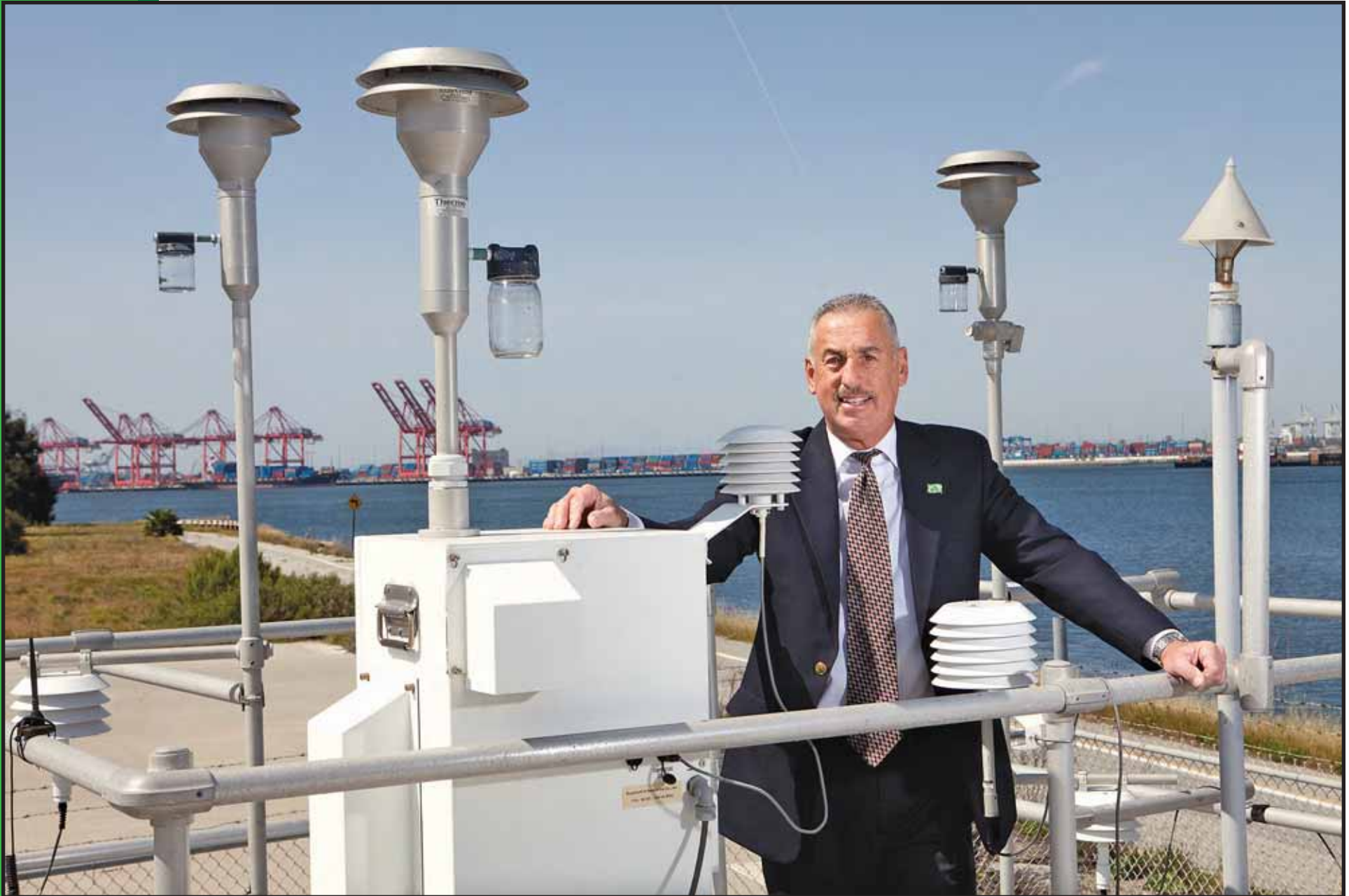
Robert Kanter, Ph.D., is the managing director of environmental affairs and planning for the Port of Long Beach. He is pictured here at one of the port's air monitoring sites located at the end of the Navy mole. The chimney-like device's are particulate matter samplers. (By the Business Journal's Thomas McConville)
