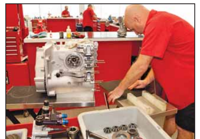
Andy Schneider puts together an Xtrac gearbox (from England) in the transmission room. The gearboxes come apart and get cleaned, inspected and rebuilt after each race.
