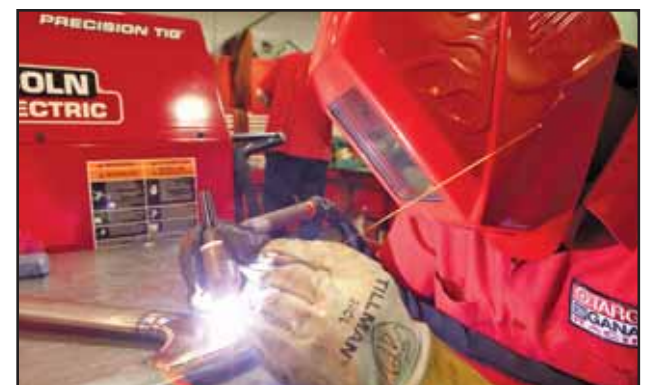
Bill Cavanaugh welds together a suspension component. Note how the tubing has been shaped for aerodynamic efficiency.
