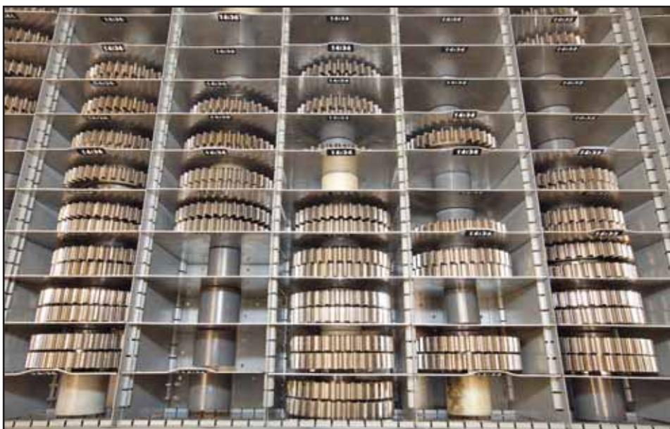
You select gear ratios for each individual track, concentrating on maximizing the drive out of each corner. Each set of six gears costs $750 or so, and is replaced after practice on Saturday at every race. Let's see, that's $750 x 17 races x two cars . . .
