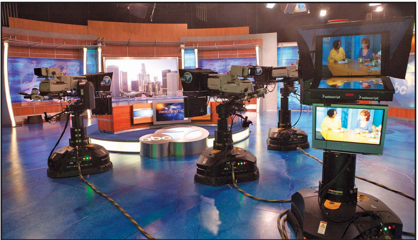
The modern news anchor set. When a Long Beach Business Journal writer visited, a live news broadcast was going on. There were only three people in the entire room: two co-anchors and a set manager. The equipment in the room – including the cameras – are robotic, controlled by one person in another room. The anchor desk has a computer with Internet access, which the anchors can use to research stories while on the air. (Photograph by the Business Journal’s Thomas McConville)
